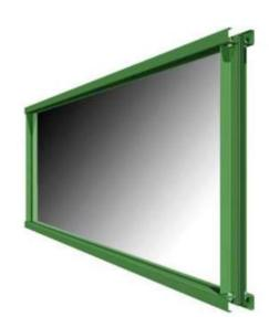
The metal sheet frame is protected from the atmospheric agents by a surface coating made of powder, with a minimum thickness of 60 microns, with subsequent fixing in high temperature oven.
